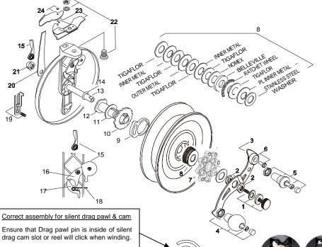
Spring loop to go over pin for correct operation of the drag.
